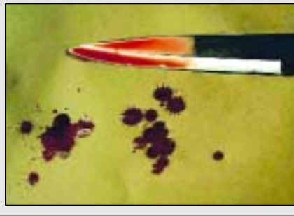
Figure 8. Classic 90° angle blood drops caused by gravity. The spines were caused by the relatively textured brown wrapping paper. Glass may have produced perfectly smooth edges.
